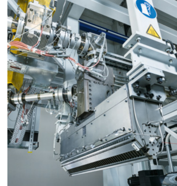
Tool unit with a melt pump, static mixer, feedblock and flat die
