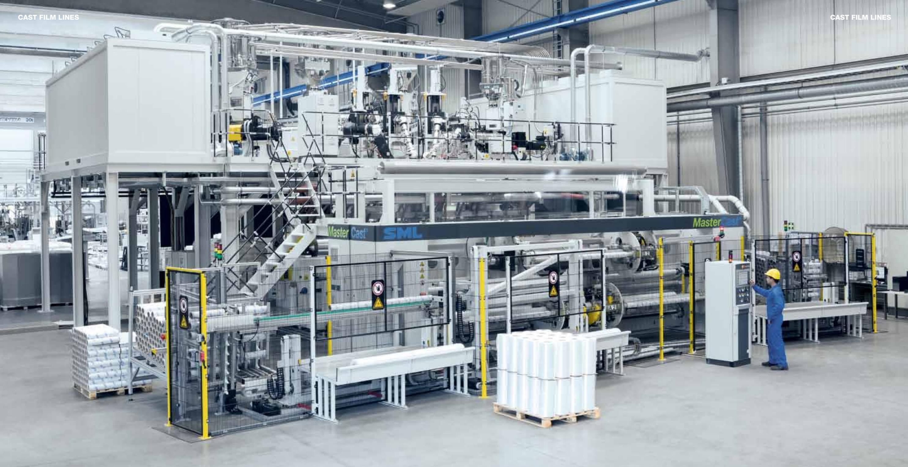
MasterCast® Stretch Film Extrusion Line
